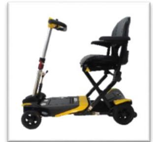
To Fold (close) the TRANSFORMER Scooter - Press and hold the A button on the key fob until the scooter is fully folded.
