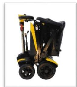
The Telescoping Tiller can be raised or lowered before or after folding or unfolding the scooter.
