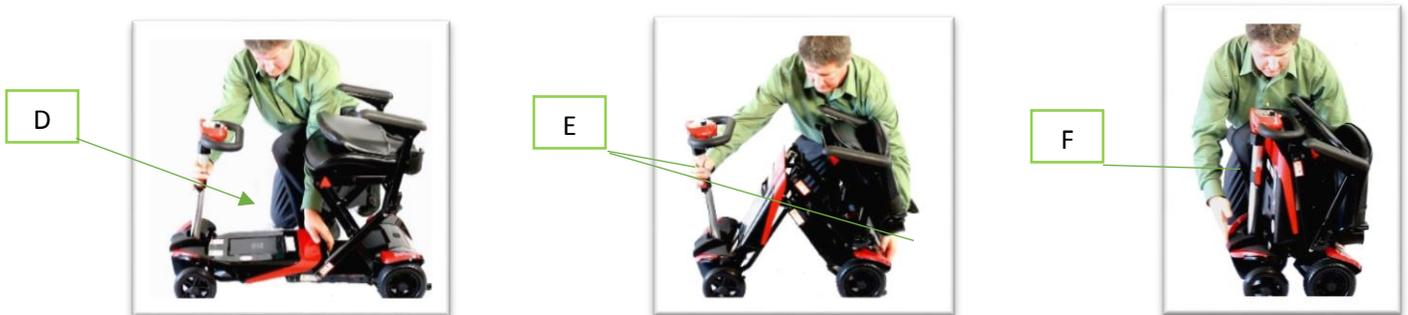
**NOTE -** If the scooter was closed by the remote control (key fob), then it must be opened by the remote control (key fob) or by using the Remote Bi-pass Switch on the back of the scooter. The manual release will not work. The scooter must be opened the same way as you closed the scooter.
