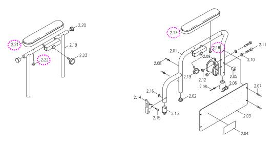
2. Use hex. tools and wrench to loosen the screw (1.08) and nut (1.05) from bracket (1.07) on the side frame (see page 14). If the armrest assembly (2.1) is worn out or deformed, then replace it.
