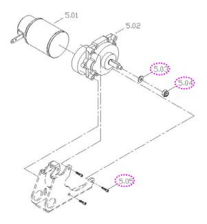
Replace the driver wheel by the following steps if it is worn out or deformed.
