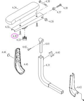
Note: The arm tube protective shrouds (4.43 and 4.45) are option parts for powerchair.
