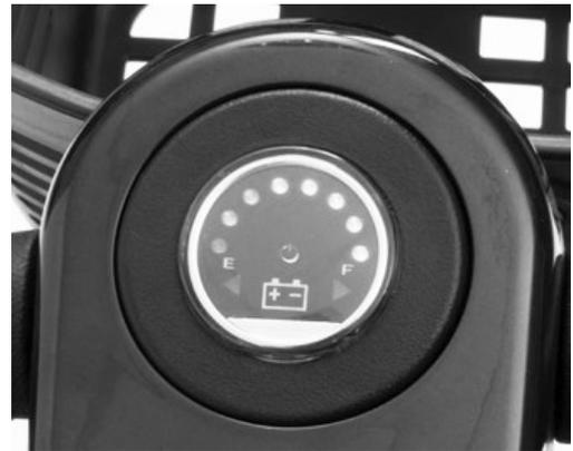
If the blue status LED located in center of the gauge is illuminated solid, then the scooter is functioning normally.
