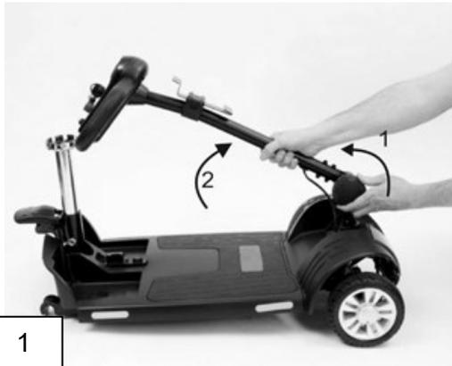
1. Raise the tiller on the front section. Turn the tiller adjustment knob towards the rear of the scooter and then lift up on the tiller by turning the knob towards the front of the scooter.
