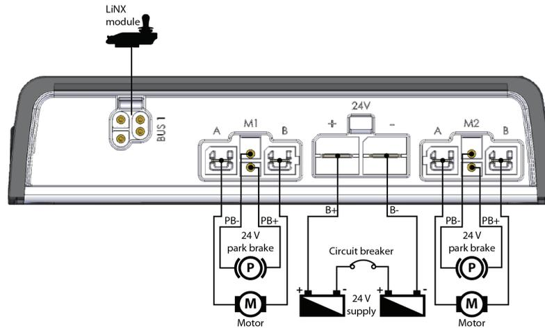
Figure 4: Typical cabling installation LiNX LE series
