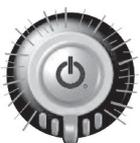
If, when powered up, there is a fault with the system, then the status indicator will flash red. The number of flashes will indicate the type of error. For flash codes, see section 10 Diagnostics.
