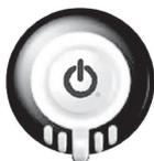
When the LiNX LE System is powered up, and there are no faults with the system, the status indicator will be lit green.
