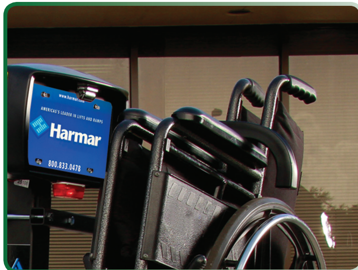
Adjustable hold-down arm safely secures wheelchair for transport.
