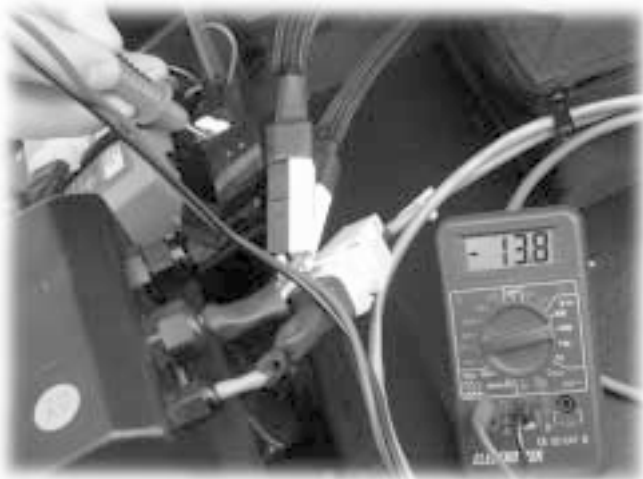
Figure 3.17. Reverse Output Voltage
