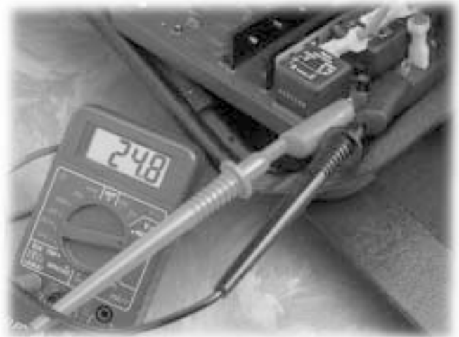
Figure 3.14. Forward Motor Voltage
