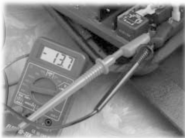
Figure 3.15. Reverse Motor Voltage
