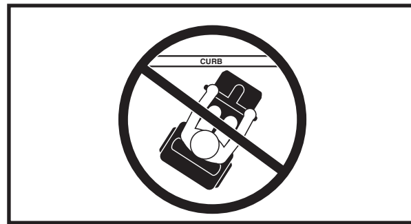
Figure 7. Incorrect Curb Approach
