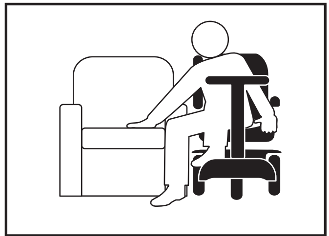
Figure 10. Recommended Transfer Position
