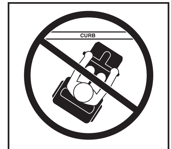
Figure 7. Incorrect Curb Approach
