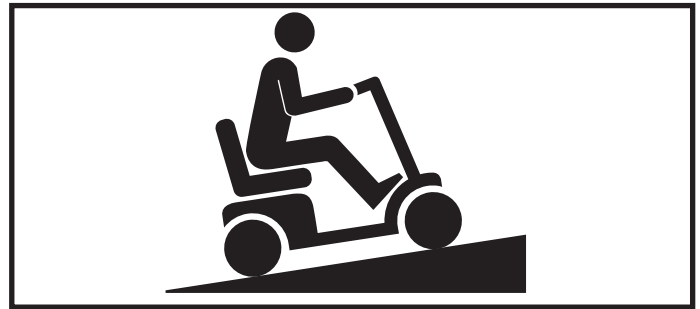
Figure 4. Increased Stability Driving Position
