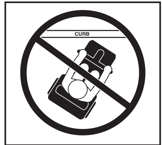
Figure 7. Incorrect Curb Approach
