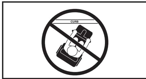
Figure 7. Incorrect Curb Approach
