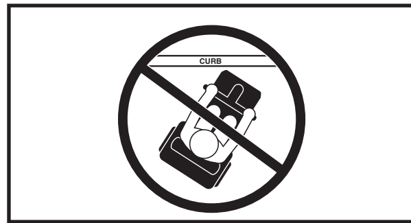
Figure 7. Incorrect Curb Approach
