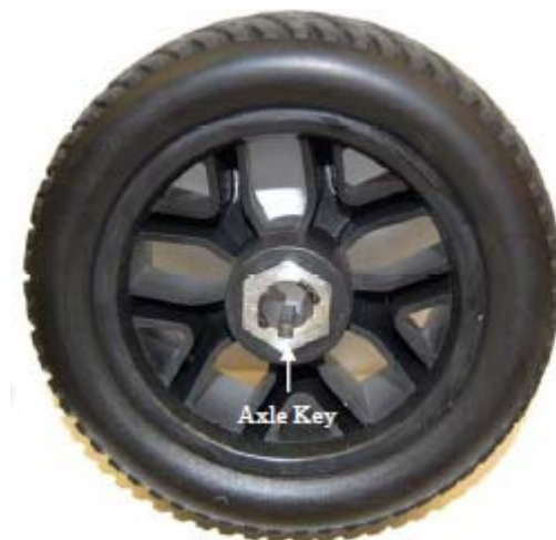
Figure 30. Drive Wheel Axle Key
