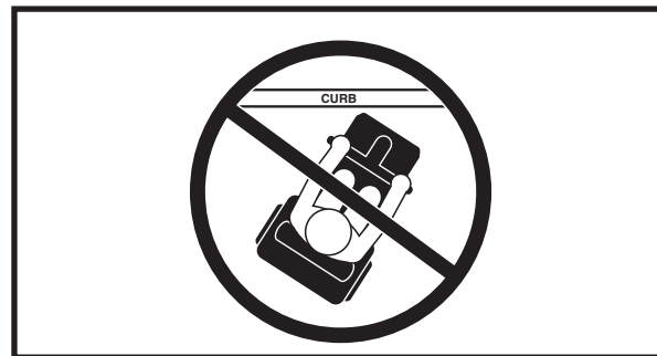
Figure 7. Incorrect Curb Approach
