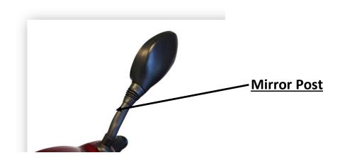
To attach the mirror simply place each mirror threaded end into the mirror post. Turn mirror clockwise and fasten mirror to scooter. Secure using a 14mm wrench on the mirror securing nut.
