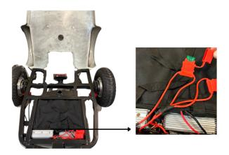
5.) After reinstalling, the battery pack put the base cover back on and rescrew the bolts to the appropriate holes.
