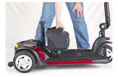
Figure 22. Battery Pack Installation
