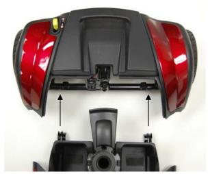
Figure 20. Drivetrain Alignment
