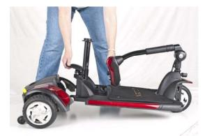
Figure 18. Separating the Drivetrain and Frame
