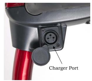
Figure 27. Charging Batteries
