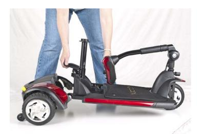
Figure 21. Connecting Frame and Drivetrain
