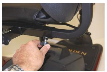
Figure 6. Armrest Width Adjustment
