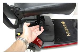
Figure 8: Seat Rotation Adjustment
