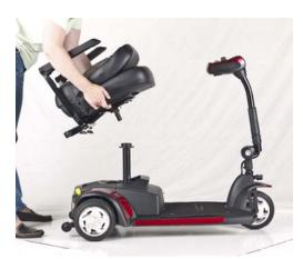
Figure 15. Removing the Seat
