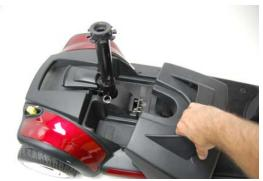
Figure 16. Removing the Battery Pack
