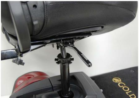
Figure 24. Installing the Seat
